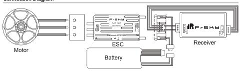
Warning: Please DO NOT connect BEC to any devices with power supply.
